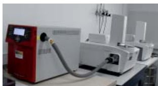
TG-DSC de Mettler Toledo+ THERMOSTAR GSD320 de PFEIFFER VACUUM
